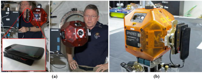
Fig. 4. 4a) Astronaut Mike Fossum testing a Smart SPHERES aboard the ISS with a highlighted image of the Nexus-S on the red SPHERES. 4b) Is a yellow SPHERES with a Nexus-S attached testing at the NASA Ames testing facility and granite table. (photo credits: NASA)
