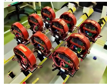
(b) Ten two-axis magnetorquers mounted on a linear air track.
